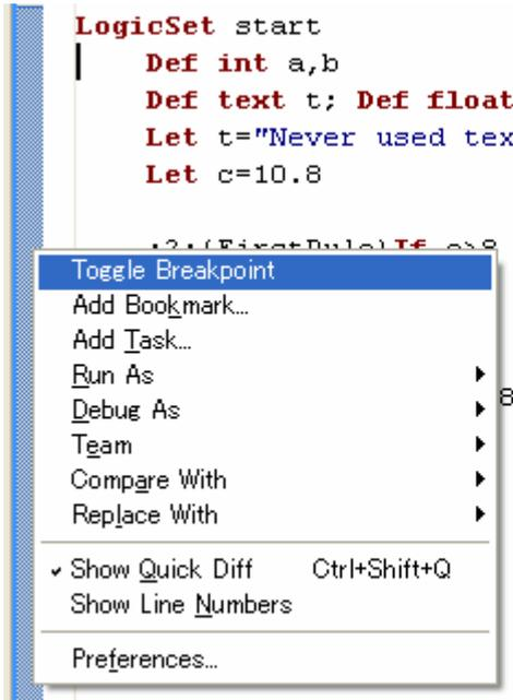
2. Double click the Marker bar before the line at which the breakpoint will be set. A blue ball is shown in Marker bar as a sign of breakpoint as below shown.
