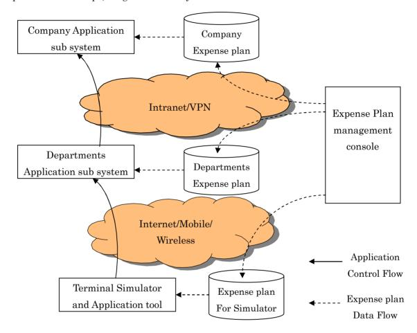
To decrease mistakes caused by plan changes, an expense plan management console is required to control all plans centrally. The console also has the functionality to broadcast plans defined to sub systems.
